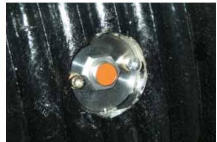
Cable drum of a mobile crane: an inductive M18 type sensor monitors and signals the cable end.
