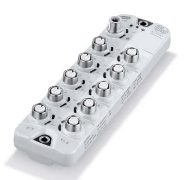
Effective connection of binary sensors to IO-Link
