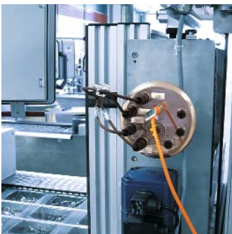
ProcessLine: St. steel module with very high protection rating in a portioning system.
