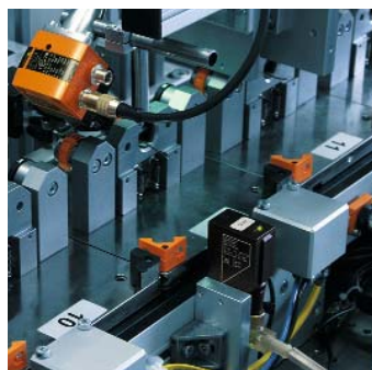
The RFID system codes and identifies workpiece carriers in a production line.
