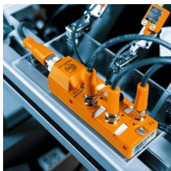
Slim, flat AS-i M8 module with tried-and-tested ecolink technology.
