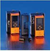
AS-Interface controllers / gateways
