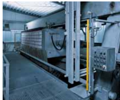
Area monitoring by means of safety light grids.
