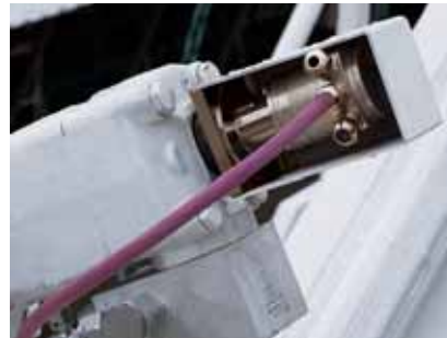
Encoder for linear measurement on a tunnel boring machine.
