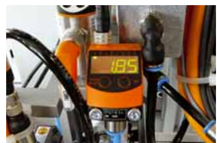
Pressure measurement in pneumatic systems.
