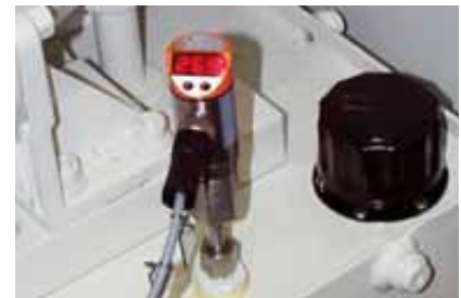
Local display of the current temperature.
