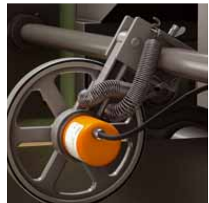
Linear measurement by means of a measuring wheel and an encoder.
