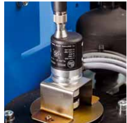
Linear measurement by means of a counter: Rotary movement is converted into digital signals.
