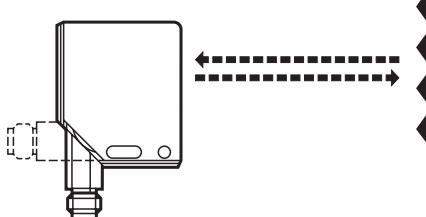
Place prismatic reflector / reflective tape in desired position. Align the photocell to a mounting bracket.
