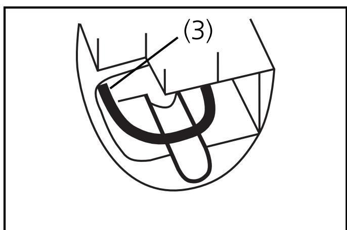
Push the connecting wires through the gland and connect the unit (see type label or page 8).
