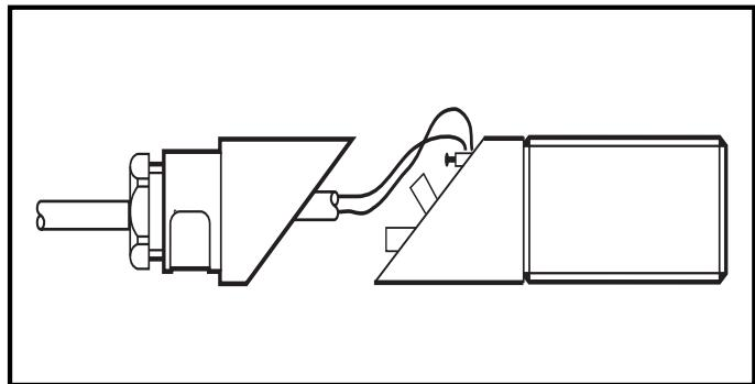
The end cap position can be straight or angled, as illustrated. Press the end cap onto the sensor accordingly and tighten the screw.
