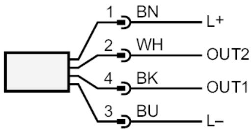
OUT1/IO-Link: switching output distance
